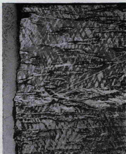
FIG. 13. The microstructure of 9% Sn-bal Bi specimens tested to failure at atmospheric pressure, 50 \times , Unetched, polarized Light.
